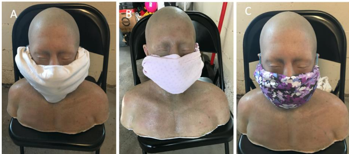
Figure 2. Photos showing the wearing of home-made cloth coverings. A) white 100% sweater, B) 100% cotton dress, and 3) 100% polyester scarf.
