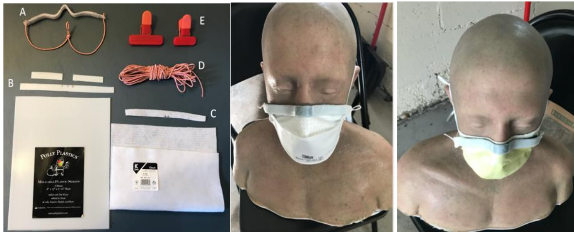
Figure 4. The major parts of the plastic nose clip and the photos showing how the nose clip is worn on top of a Aura N95 respirators and an HIS surgical mask for improving the fit of the mask to the face. The items listed in the left photo: A) the complete plastic nose clip, B) pieces cut from a heat-moldable plastic sheet, aligned for making the external nose clip, C) a felt strip cut from a felt sheet, D) elastic cord, and E) bag clips.
