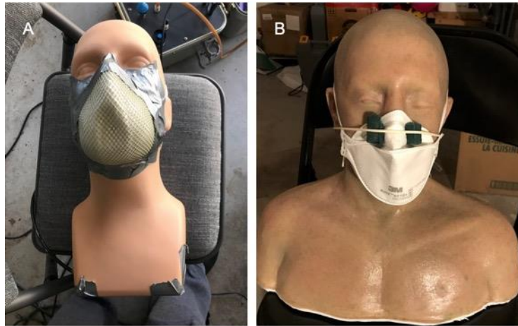
Figure 3. Sealing a Moldex N95 respirator to plastic mannequin with duct tape (A) and a 3M mask modified by using an additional elastic band and rolls made from a kitchen scouring pad to press the mask on either side of the nose of the silicone head (B); this was the inspiration for the customized nose clip.
