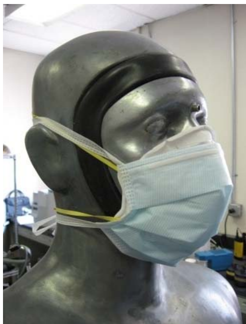
Figure 1. Smartman breathing mannequin with a N95 filtering facepiece respirator and surgical mask affixed.
