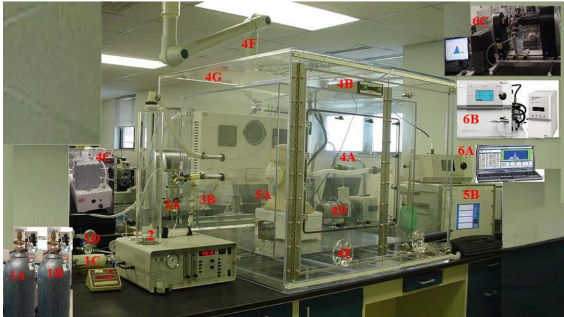
Fig. 1. The bio-aerosol respirator testing system: compressed air supply (1A); nitrogen air supply (1B); HEPA filter (1C); air flow regulator (1D); VOAG (2); nebulizer (3A); nebulizer dilution air inlet (3B); exposure chamber (4A); temperature and RH controller (4B); Ultrasonic Humidification generator (4C); exhaust port with HEPA filter (4D); ventilation air inlet (4E); ventilation air outlet (4F); a secondary containment (4G); a head form with a FFR (5A); breathing simulator (5B); APS system (6A); SMPS system (6B); and Spraytec Laser system (6C).
