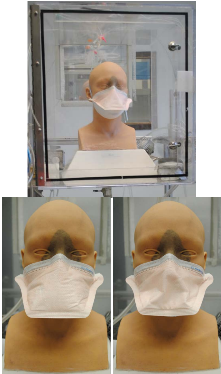
Figure 1a. A flat fold respirator (Kimberly Clark 46727) mounted on a headform at no breathing condition inside the test chamber (Top).
