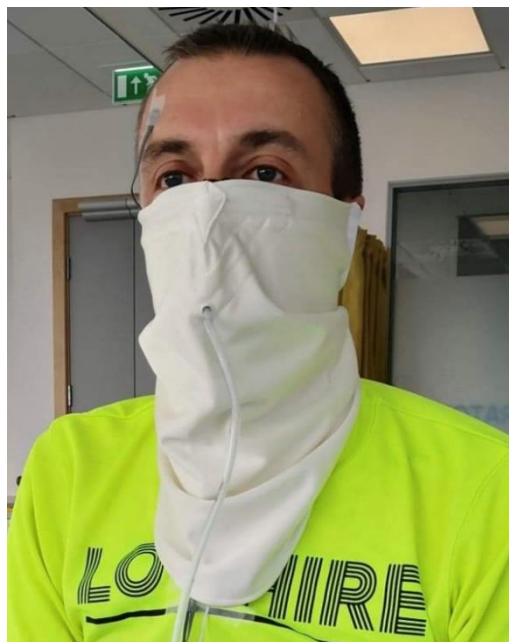
Figure A: Participant wearing a then-prototype cloth mask, a facegaiter™ (tensARC, Stirling, UK) mask with bespoke attachment (A) to sample gas composition inside the mask and visible skin thermistor on the forehead (B). Photograph used with participant's permission.
