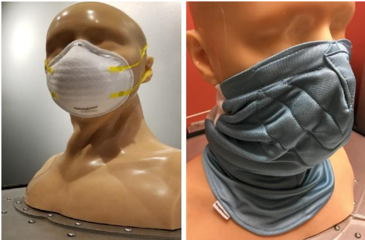
Figure 3. Dynamic head form having silicon skin, with control on left (N95) and the tubular face mask (Filter A) on right, utilized to gauge whether there was consistent “whole mask” performance as worn.
